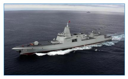
Unlike the nearly completely smoothed over Zumwalt class deck and hull structure, the Chinese Type-055 does have DDG 51-like protruding antennas on its back half, something which could reduce its stealth properties by virtue of being vertical structures likely to be detected by radar return "pings" and also emit a potentially detectable electromagnetic signature.
